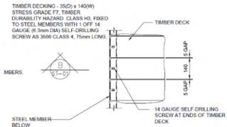
The platform should be large enough to support all edges of the tank. With reference to the picture above, the recommended gap between the timber decking boards is 5 mm and must never be greater than 25mm. The tank stand is required to be level with no more than a 1°slope.
