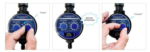
1i. Ensure that the reset interval and drain time knobs are in the "RESET" and "CLOSED" positions. Set your reset interval and drain time according to the tables in Figure 2, then replace the battery box cover.
