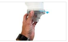
1c. Attach the Advanced Release Valve by first installing the 25mm x 20mm (1" x 3/4") reducing adaptor and washer to the 25mm (1") thread of the screw cap.
